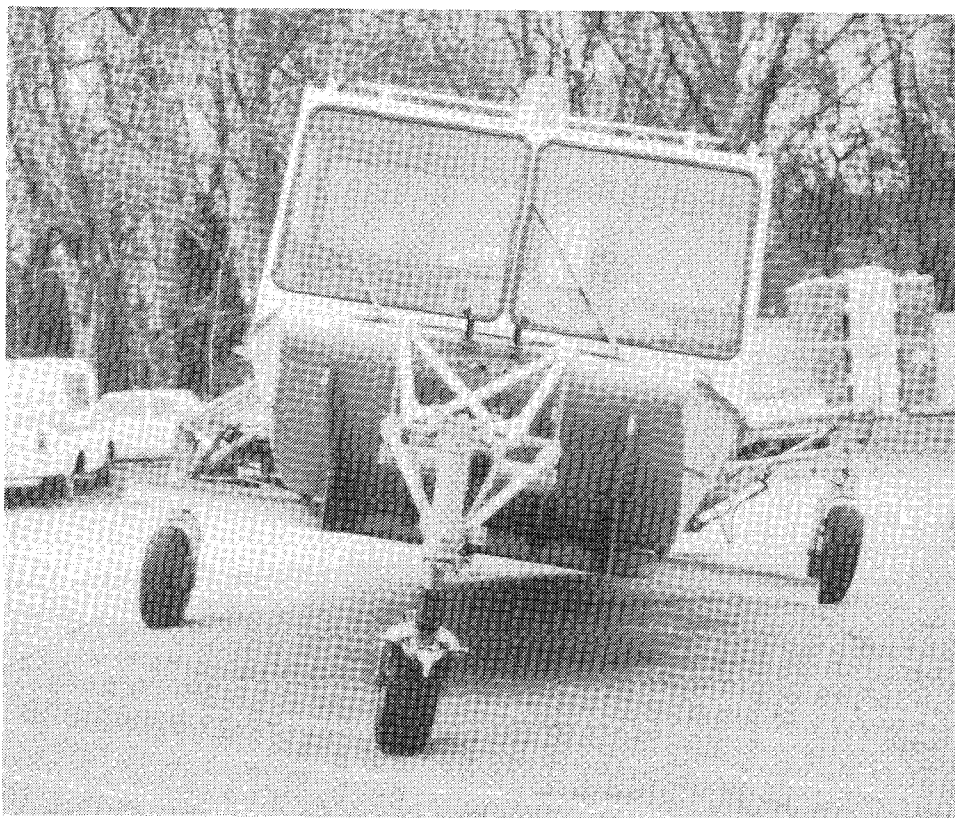
Fig. 2 Airboat test frame for tilt steering research.
